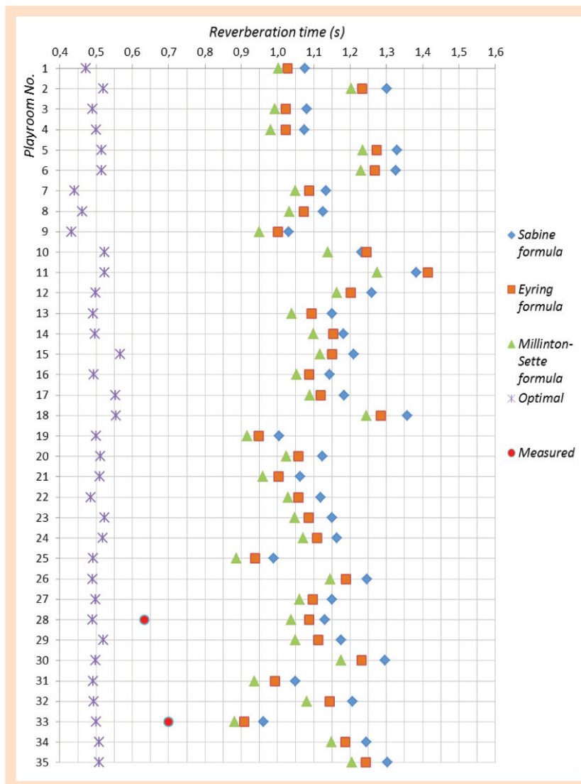
Figure 1: Calculated, measured and optimal reverberation times [s] in 35 playrooms of 16 kindergartens.
