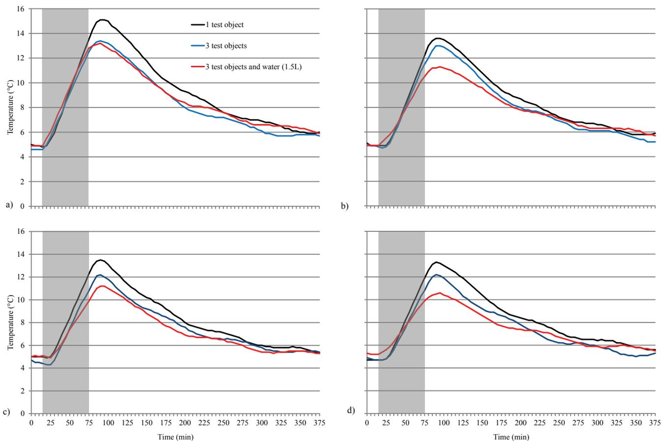
**Figure 2:** Comparison of internal temperature movement of test object at 30°C external temperature and different internal conditions in a) bag 1, b) bag 2, c) bag 3 and d) bag 4. The grey area indicates the time period (60 minutes) when the insulated bag and its content were exposed to controlled outside temperature.
