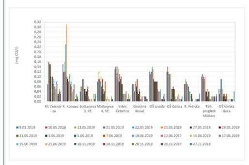
A gradient of free chlorine concentration reduction at the water supply system in the direction of water flow from the chlorination reference point to the farthest chlorine measurement location was constructed (Figure 5). The trail from R1 Velenje to OŠ Vinska Gora represents a distance of more than 9 km.
