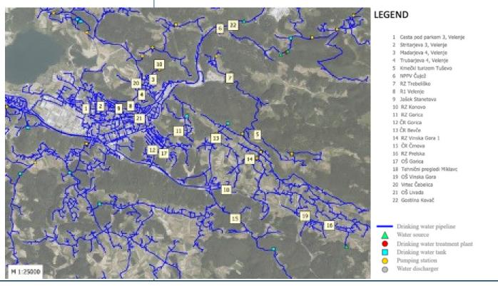
Water sampling was performed by Komunalno podjetje Velenje before and after water treatment, at water reservoirs, on the network and at the taps of fifteen users (residential buildings, schools, kindergartens, companies). The measurements for free chlorine and measurement of microbiological parameters were conducted twice a week in two months (May-June 2019).
