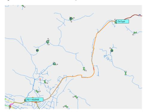
The selected supply area represents 45 % of all users, 25 % of the total volume of the water supply network and 35 % of the average daily distributed quantity of drinking water in the entire water supply system of city of Velenje. The systematic sampling of water was conducted at 22 pre-defined measuring points (Figure 3), which were distributed throughout the supply area at intermediate water supply facilities and at the outlets of end users.
