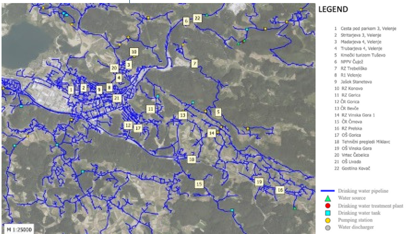
Figure 3: Selected sampling points at R1 Velenje for measurement of chlorine concentration and microbiological parameters.
